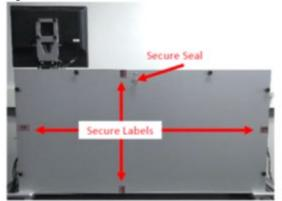
(c) On the right side of the DS450, a clear access door protects the USB ports. The access door must be secured using the integrated key lock, a label seal, and a wire or padlock seal; and
