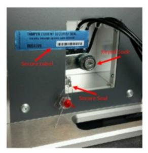
(d) On the left side of the DS450, a clear access door protects the power switch, power cord, network port, and USB port. The access door must be secured using the integrated key lock and a wire or padlock seal. A label seal must also be applied any time the access door is opened and closed again; and
