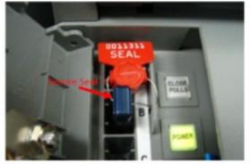
(b) Close the access door and lock with a medium barrel key. Affix a label seal over the place where the access door meets the body of the machine;
